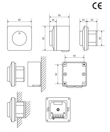
Output current: Rated voltage PRI: Rated power: 0,25 - 2,5A 230V 50/60Hz 80 - 460W
