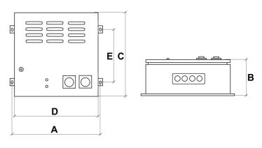
Rated current SEC: Rated voltage PRI: Control type: 1,5 - 14A 3 x 400V 50/60Hz 5-step regulation
