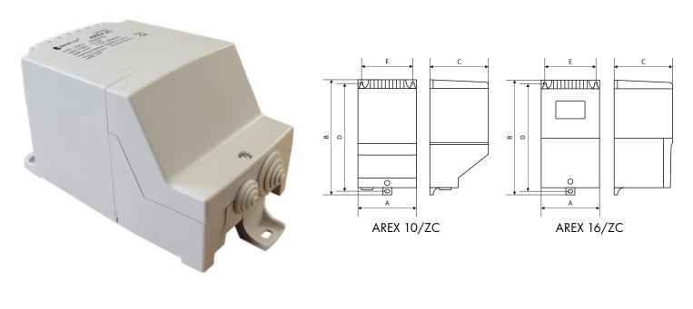
Output current: Rated voltage PRI: Range of output voltage: Control type: 10A; 16A / 13A 230V AC 50/60Hz / 3 x 400V 50/60Hz 0 - 230V AC / 0 - 400V AC (50 degrees of control) 0 - 10V DC, 0-20mA, MODBUS RTU
