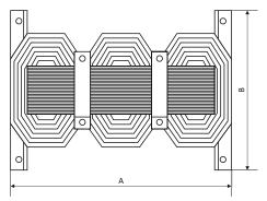
Rated power: 10 Rated voltage PRI: 100 Rated voltage SEC: 24 Winding: AI,
