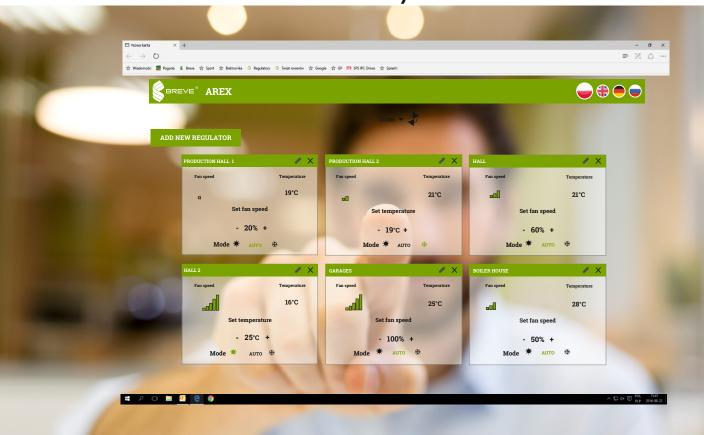
RegiSoft system is based on AREX/A fan speed regulators with MODBUS protocol and dedicated software for PC computers
