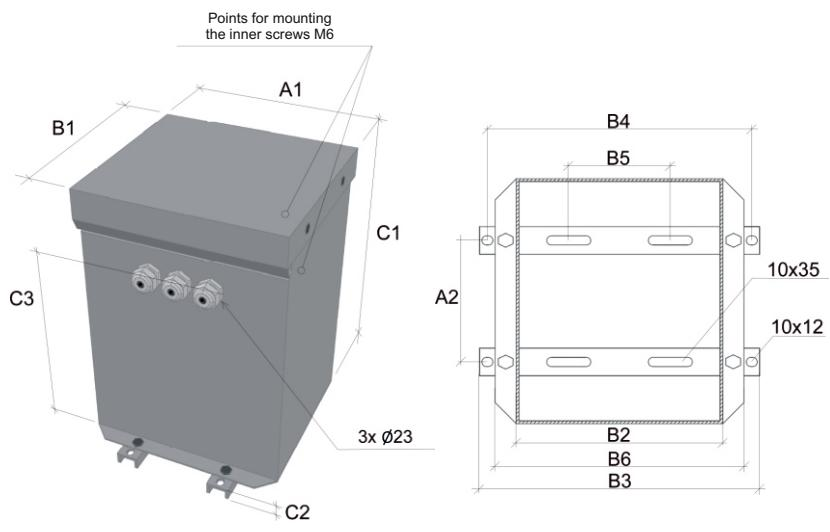
UMD/2 transformers could also be delivered in B1U housing with IP23 protection grade. Thermal class for transformer and housing set is 30°C.
