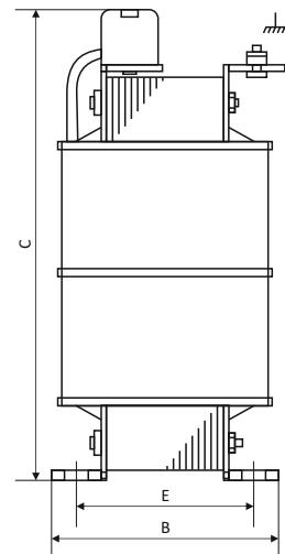
Insulation Test voltage: **4,0kV 50/60Hz**
